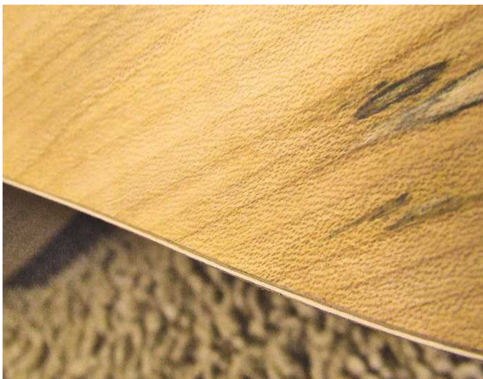
▲ Pic.24 Here's a close up of the body binding – layers of veneer, comprised of walnut, maple, then walnut again. It's a tiny detail but the effect is impressive
